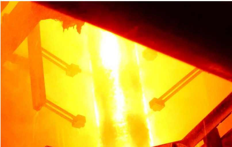
Fig. 3: “Black stripes” on round billet as a result of non-uniform spray nozzle cooling
